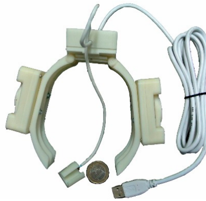
Figure 5. Prototype implementation of the assessment system (glove part) for parkinsonian motor symptoms. In addition to tremor assessment, this modified version of the assessment system can be used to assess bradykinesia, dyskinesia, and rigidity.
