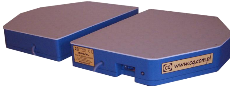
Picture. 1. Two platform stabilographical scale of „CQ Elektronik System” [7]
